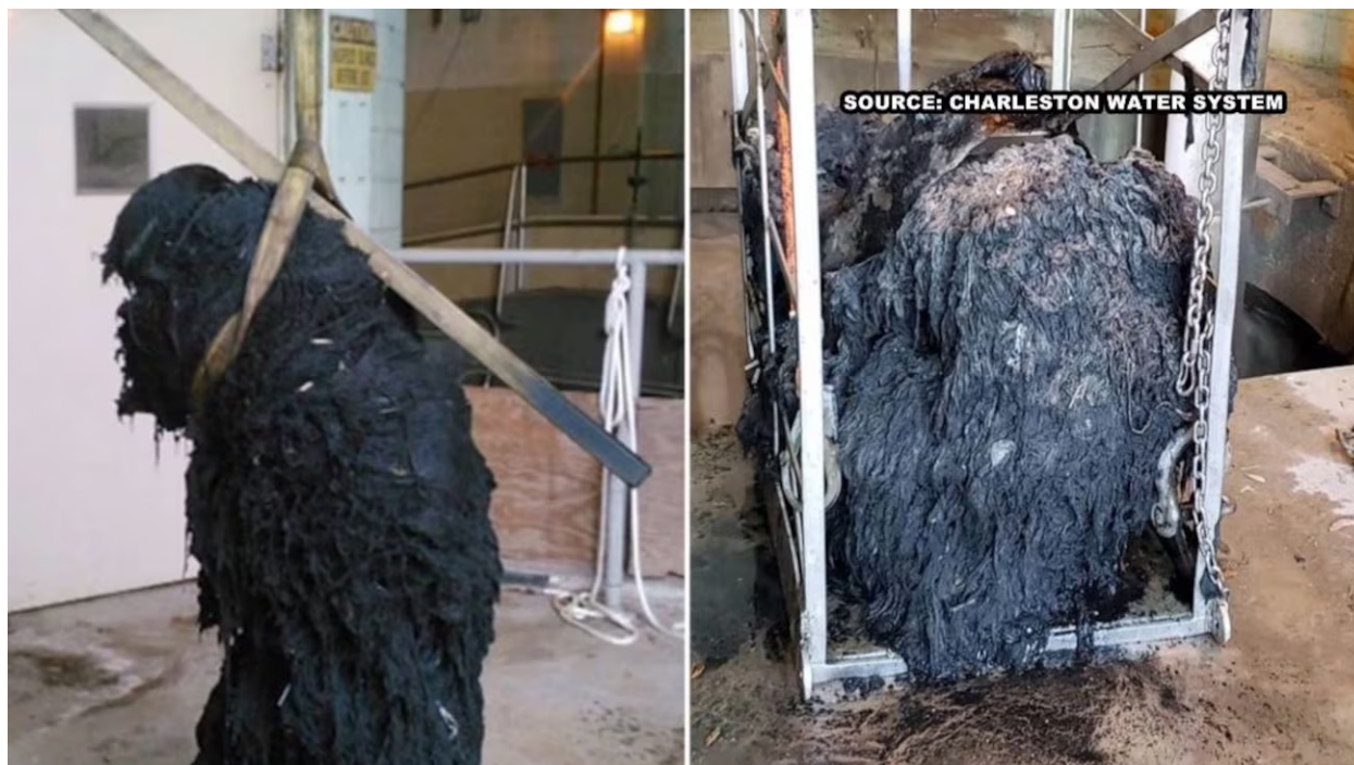
FIGURE 7: “FLUSHABLE” WIPE CLOG
