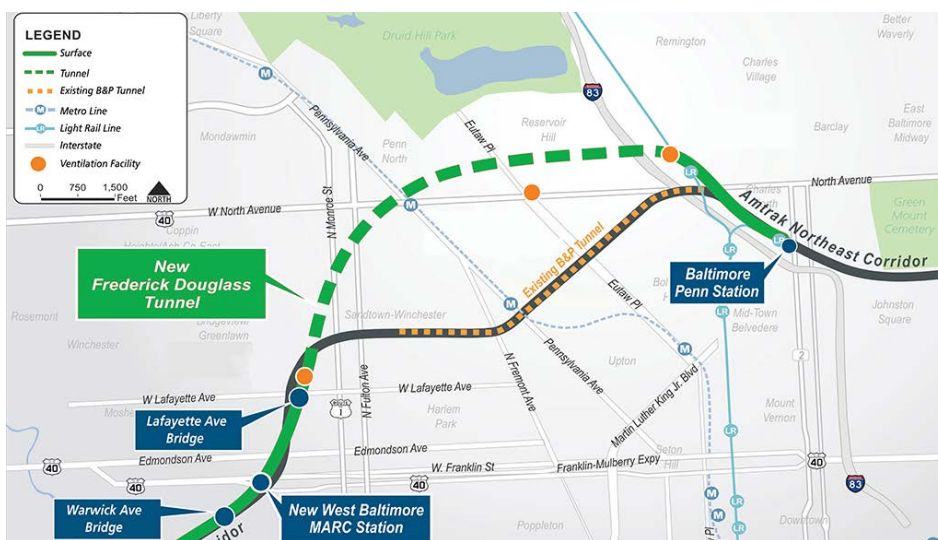
Figure 2. Frederick Douglass Tunnel improvements
