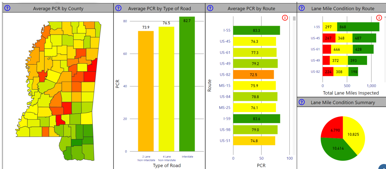
FIGURE 1: PCR FOR INSPECTED ROUTES IN MISSISSIPPI
