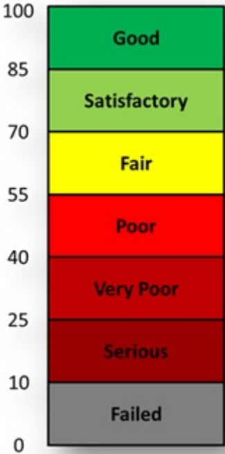
FIGURE 2. PAVEMENT CONDITION INDEX (PCI) RATING SCALE FOR ASPHALT CONCRETE (AC) AND PORTLAND CEMENT CONCRETE (PCC) PAVEMENTS (Courtesy of FAA PaveAir).
