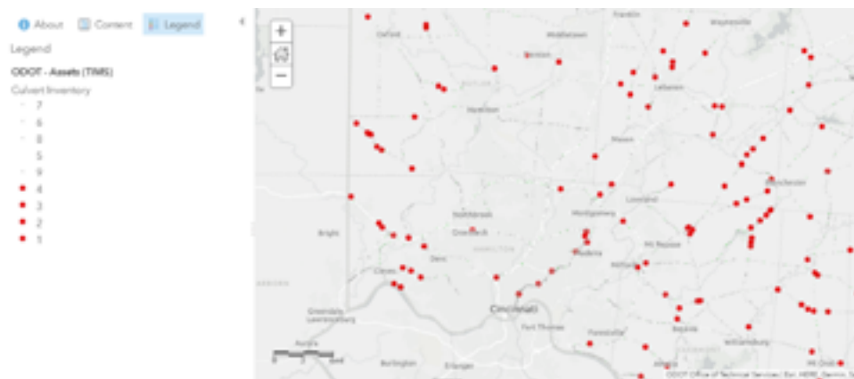
FIGURE 5: ODOT CULVERTS AT AN UNACCEPTABLE STRUCTURAL CONDITION (RATINGS 1 TO 4) IN SOUTHWEST OHIO
