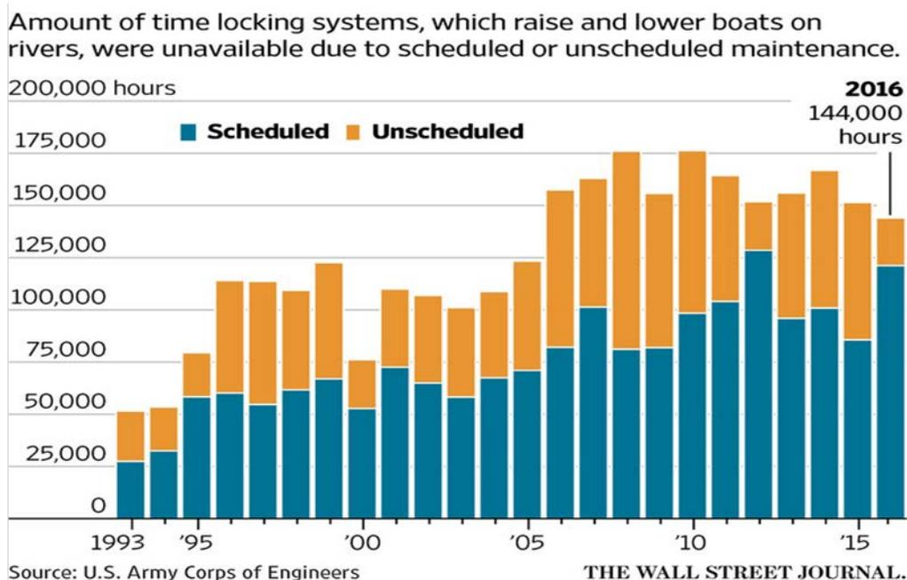
Figure 3: Lock Closures for the Ohio River, Illinois Rivers and the Upper Mississippi River
